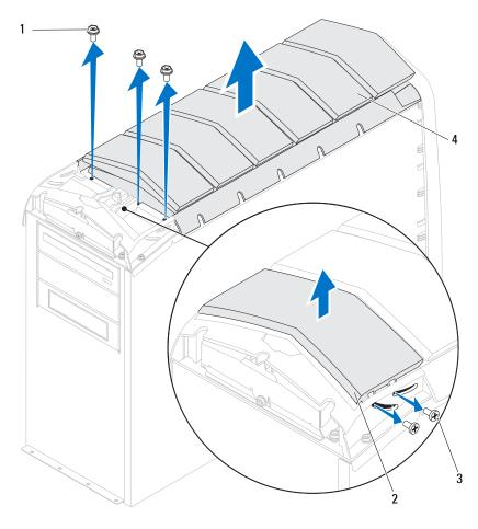
1top-vent screws (3)2top I/O panel cover3top-panel screws (2)4top vent
